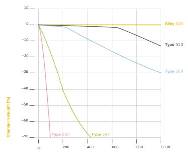
Hours of Cyclic Exposure (15 mn Heating, 5 mn Cooling)
